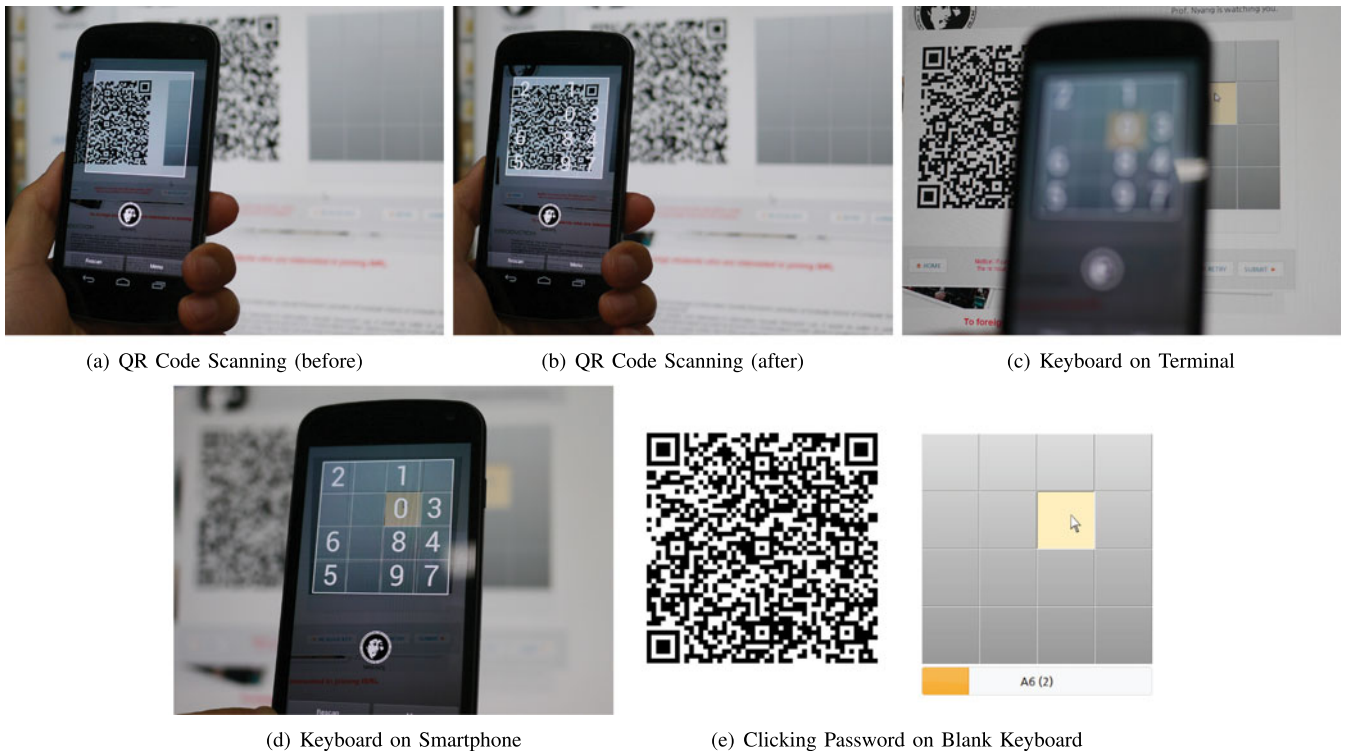
Fig. 2. Photographs of the prototype we have developed to demonstrate our authentication protocols. (a) and (b) show the moments of a QR code scanning of a keyboard layout. (c) shows the blank keyboard shown at the terminal (on LCD screen). (d) shows the decoded randomized layout of the keyboard obtained from the QR code after decryption as viewed on smartphone. Note that the yellow square on which the mouse cursor is hovering in the terminal is shown through the smartphone to assist user’s input. (e) shows that a user is clicking the password on the blank keyboard while seeing numbers through the smartphone.
